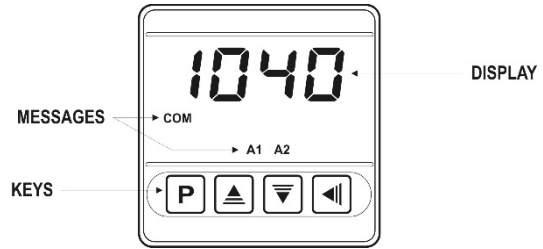
Figure 6 – Identification of the front panel parts
