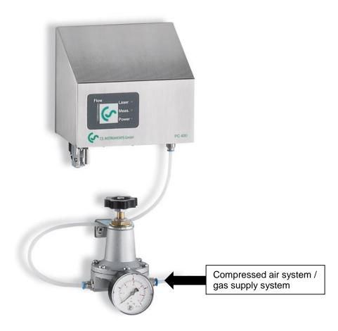
Important: The pressure at the particle counter PC 400 is not allowed to exceed 1.6 bar overpressure. The pressure has to be reduced correspondingly by means of the supplied pressure controller.
