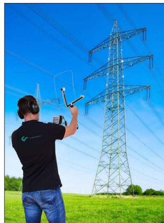
Checking high-voltage overhead lines for corona discharge
