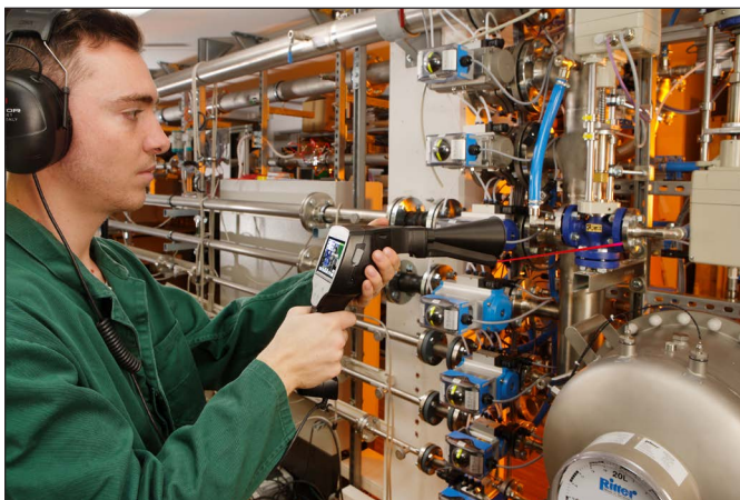
Accurate leak detection during operation with laser pointer and integrated camera
