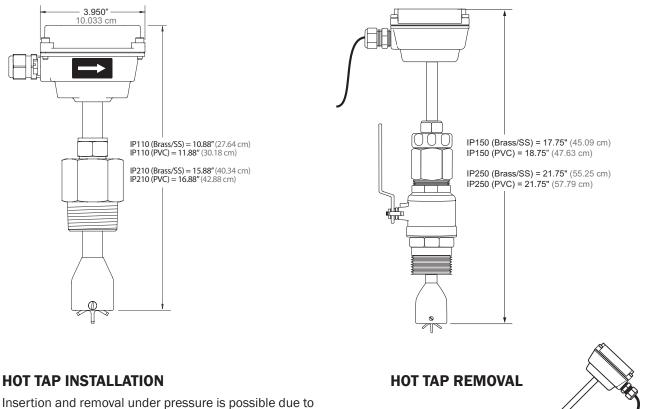
Insertion and removal under pressure is possible due to the 2" full-port isolation valve, which comes with a nipple for installation on the pipe fitting. If it is necessary to do the initial installation under pressure, any standard hot tap drilling machine with 2" NPT adapter, such as a Transmate or a Mueller, can be used. Ordinarily, it is not necessary to use an installation tool, since the smalldiameter tube can be controlled by hand at all but the highest pressures.
